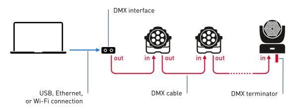
Each daisy chain of fixtures forms a **DMX universe** which operates up to 512 channels. For many installations a single universes is sufficient, but Lightkey can control up to eight full universes or 4096 channels.
