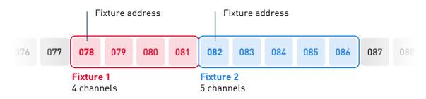
Some fixtures have a DIP switch (Dual In-line Package) for setting the address as a binary number. Other fixtures have an on-device menu. See the documentation that came with your fixture.
