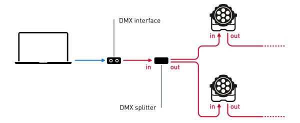
Other equipment includes **DMX boosters**, which amplify the signal over long cable runs, and **DMX transmitters**, which transmit DMX wirelessly. From Lightkey's perspective it doesn't matter if you employ splitters, boosters, transmitters, or cable adapters along the DMX line. The software does not specifically control those devices and doesn't even know they're there.
