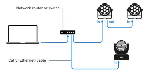
Some network-enabled fixtures can also route the Art-Net or sACN input to their XLR out port, so you can connect more fixtures with DMX cables. The exact capabilities depend on the fixture; please refer to the fixture documentation for details.
