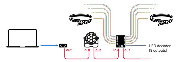
Some more advanced fixtures have RJ45 (Ethernet) ports and can receive data directly from the computer or through an Ethernet router or switch using network protocols like Art-Net or Streaming ACN (sACN or ANSI E1.31). Most of these fixtures also have an RJ45 out port so they can be daisy-chained.
