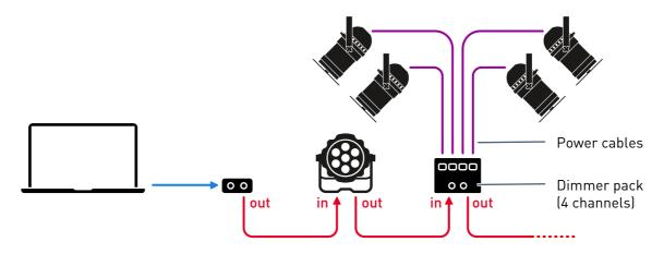
You can connect digital LED strips through a DMX-compatible **decoder** which translates DMX to a PWM (pulse-width modulation) signal for controlling the LED colors. Most decoders control multiple LED strips at once.
